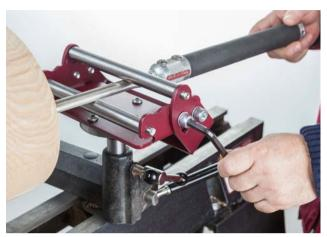
Slacken the cantilever locking screws and adjust the upper roller until it sits securely on the top of the tool shaft and lock into position
