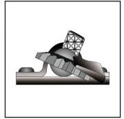
Use a diamond file or honing stone to sharpen the top bevelled face of the cutter. Slowly rotate the cutter while rubbing the stone or file across the bevelled face keeping it at the same angle at all times.
