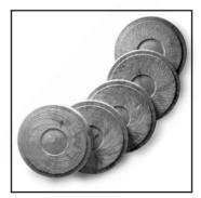
A huge variety of patterns and textures can also be produced by using the points and edges of the teeth and by changing the speed of the lathe.
